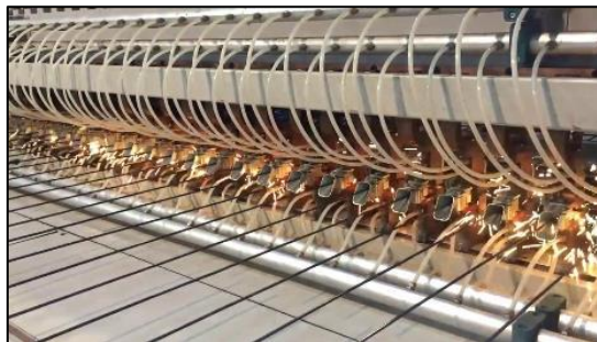
Figure 5.29: Illustration of welding process
